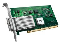
Using the Intel PRO/10GbE SR Server Adapter, enterprises can cost-effectively deploy 10GbE to a broad range of servers using lower-cost multi-mode fiber optic cabling and switching infrastructure. The 10GbE SR standard enables 10GbE transmissions at distances up to 300 meters using standard multi-mode cabling.
